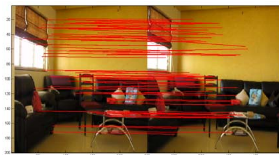
Fig.4: Features detected by Scale Invariant Feature Transform (SIFT) and matched by using nearest neighbor algorithm
