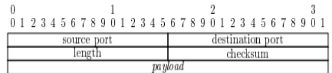
Figure 3.4: The UDP header structure [Pos80].
