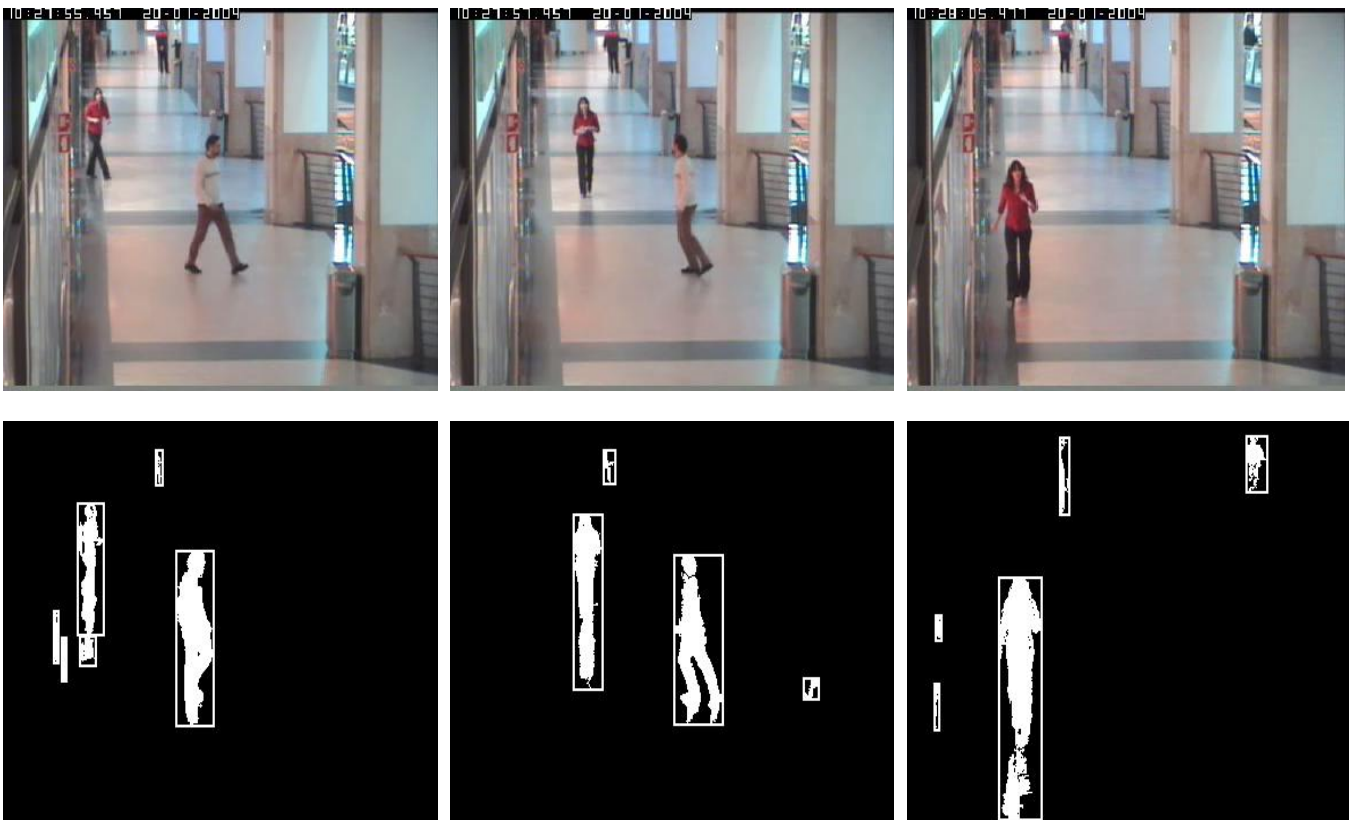
Figure 3 Top row shows original frames (frame no. 150,200,388) CAVIAR [11] database sample (indoor). And bottom row shows detected objects
