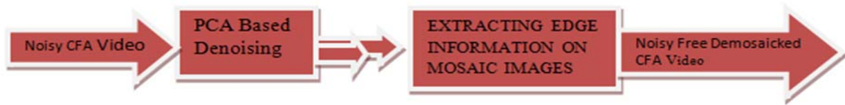
Fig. 2. Two stages of the proposed video denoising and demosaicking scheme for noisy CFA video
