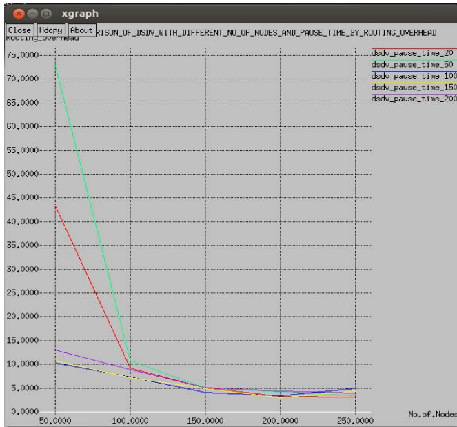
Fig. 3 routing overhead for DSDV for different pause time and number of nodes
