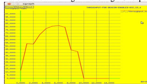
Fig. 12. Throughput vs BO=SO in Star Topology in Beacon- Enabled Mode
