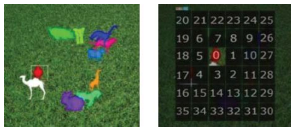
Fig. 4. A ClickAnimal image (left) and 6 \times 6 grid (right) determined by red turkey’s bounding rectangle.
